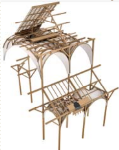
Left: model of the bearing structure Above: detail of the structural strengthening devices. A complex system of steel tie rods was designed through mathematical modeling to strengthen the trusses and top structure.
