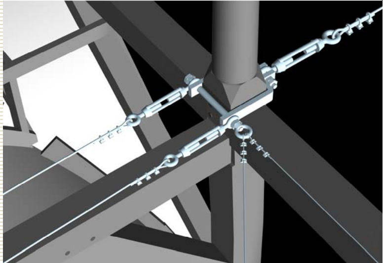
Left: model of the bearing structure Above: detail of the structural strengthening devices. A complex system of steel tie rods was designed through mathematical modeling to strengthen the trusses and top structure.
